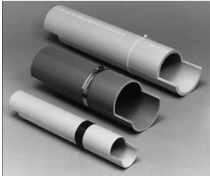
The fast and easy method of installing duct around existing cable for repair and temporary installations.
